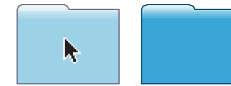
Figure 3-4. The effect of the changing alpha values using mouse over and mouse out events
